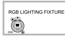
DMX FIXTURE WITH RJ45 CONNECTORS **TYPICAL APPLICATION - PERMANENT & TEMPORARY INSTALLED FIXTURES.**
